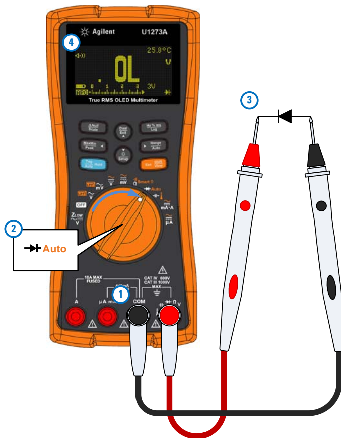
Figure 2-21 Testing a reverse-bias diode
